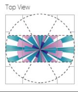
If necessary, the masked area can be altered by cutting off the respective grooved segments with a wire cutter or knife.
